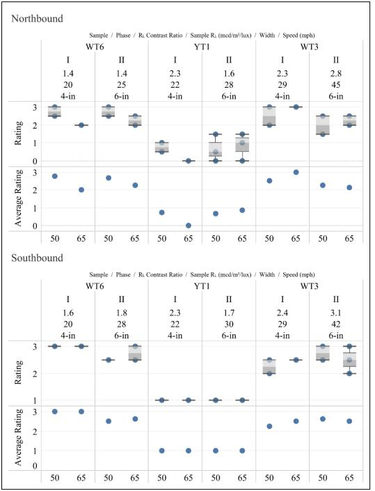
Figure 26 presents the observations of the Phase II 6-inch-only samples and their Phase I 4-inch comparison markings, during dry, nighttime conditions. Once again, no discernible effect of speed can be identified. Only two speeds were used in the data collection (50 and 65 mph).
