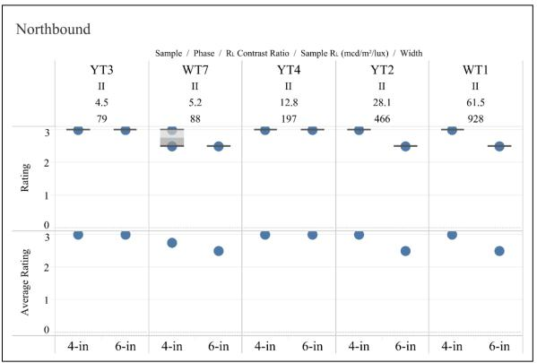
Figure 42. Dry, Nighttime, Glare Observations, 4- and 6-inch Phase II
