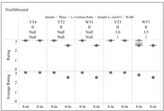
4- and 6-inch Phase II Sample vs. Luminance Contrast Ratio, Dry, Nighttime, Glare Conditions
