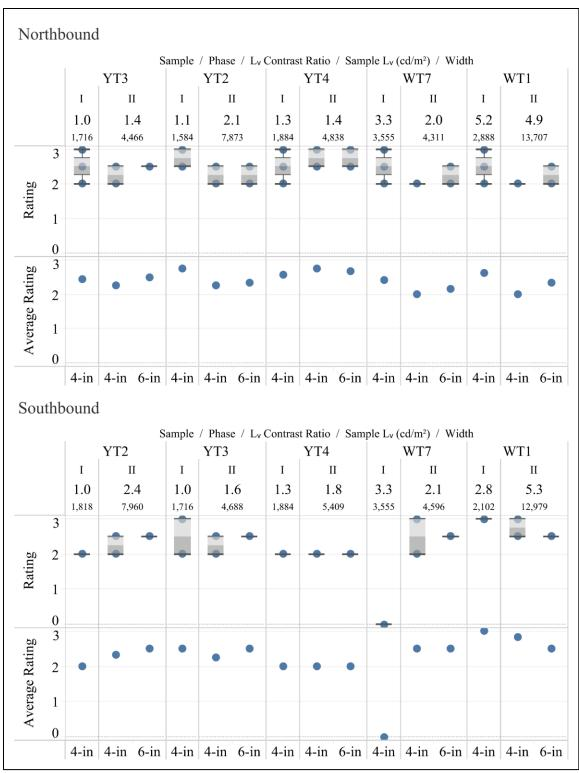
4- and 6-inch Phase II Sample vs. Luminance Contrast Ratio, Wet, Daytime Conditions
