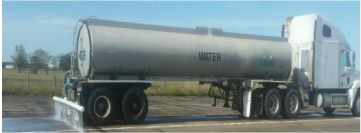
Figure 2. Water Distribution System on Semi-Trailer
