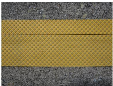
Figure 7. Example 4- and 2-inch Sections of the Preformed Tape Pavement Marking
