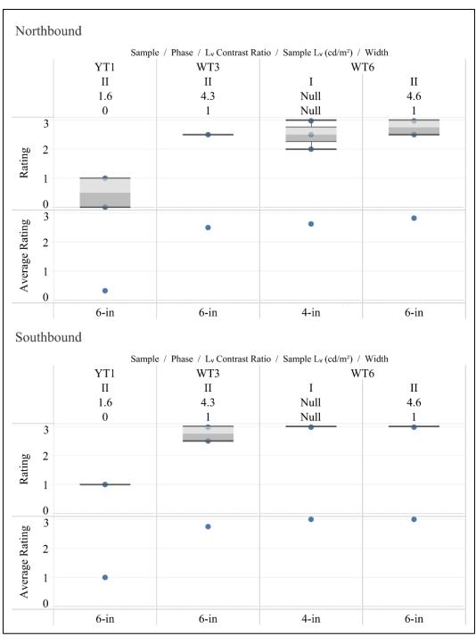
6-inch Phase II Sample vs. Luminance Contrast Ratio, Wet, Nighttime Conditions
