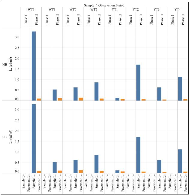
Figure 18. Phase II CCD Luminance During Wet, Nighttime Conditions
