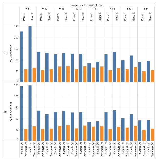
Figure 9. Retroreflectometer Qd Measurements
