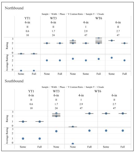
Figure 30. Phase II 6-inch Markings Wet, Daytime, Cloud Cover Assessment
