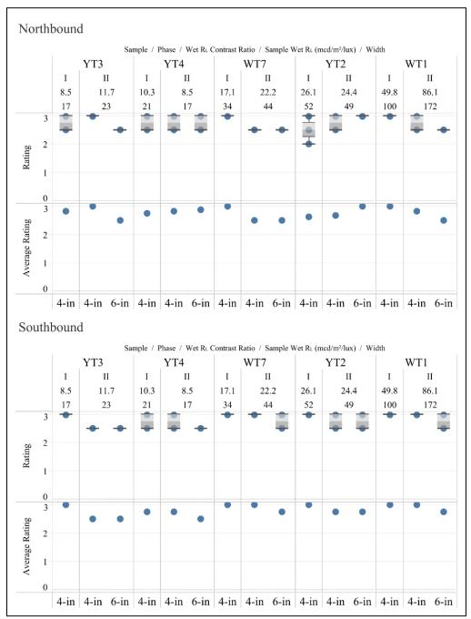
Figure 40. Wet, Nighttime Observations, 4-inch Phase I vs. 4- and 6-inch Phase II
