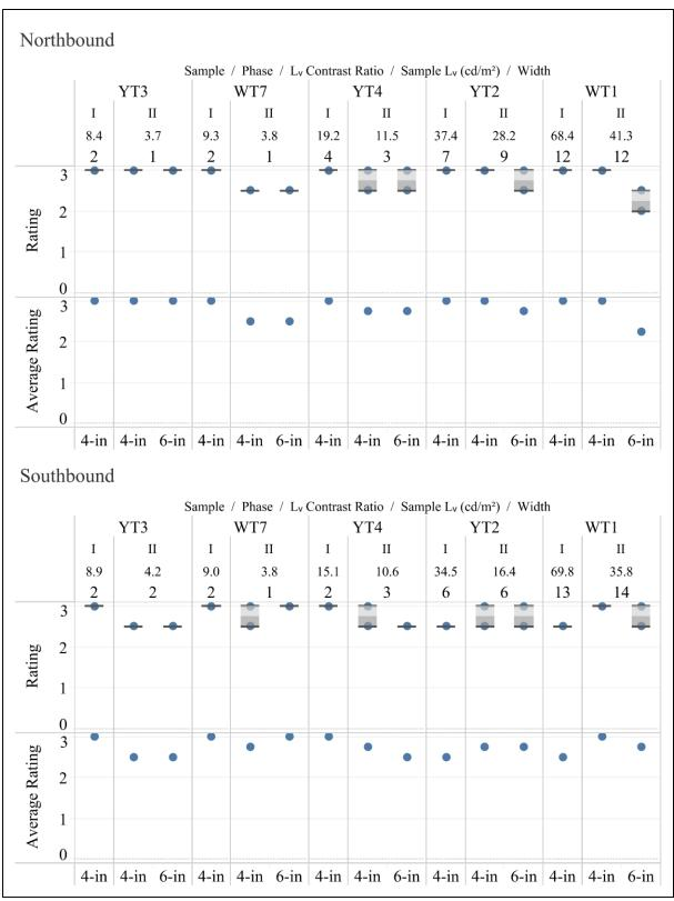
4- and 6-inch Phase II Sample vs. Luminance Contrast Ratio, Dry, Nighttime Conditions
