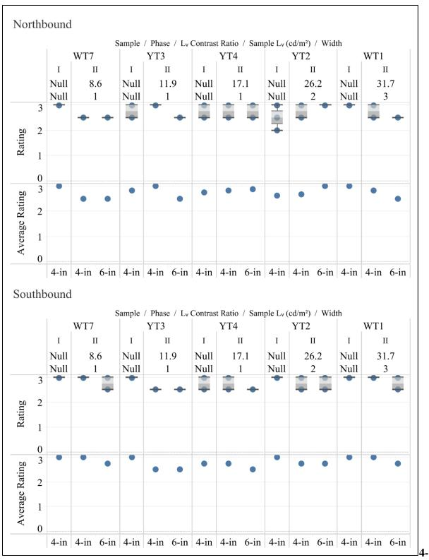
and 6-inch Phase II Sample vs. Luminance Contrast Ratio, Wet, Nighttime Conditions
