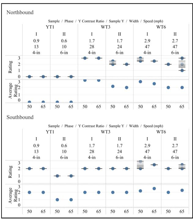
Figure 24. Phase II 6-inch only Markings by Observation Speed, Dry, Daytime Conditions
