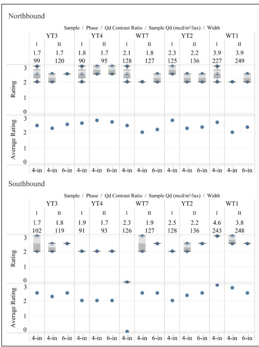
4- and 6-inch Phase II Sample vs. Qd Contrast Ratio, Wet, Daytime Conditions
